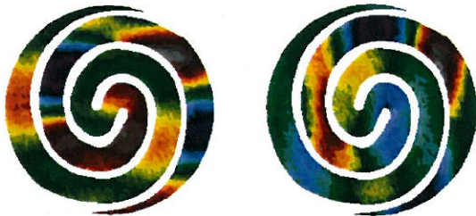
Fig. 6: Vibration mode of catalytic converter at 2364 Hz: the colors indicate direction and amplitude of the vibration in horizontal (left) and vertical direction (right)
